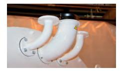
Liquid infeed pipes and 150mm ventilation fan at gearbox end, replaces previously supplied hopper.
