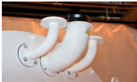
Liquid infeed pipes and 150mm ventilation fan at gearbox end, replaces previously supplied hopper.
