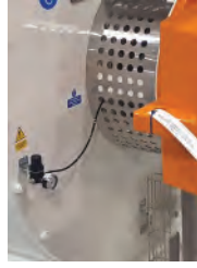
Pressurized Air Chocolate Seal for leak free solution at gearbox end. No gland packing.
