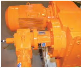
Linear "no contact" transducer to monitor position of pressure system, creating a virtual pressure scale viewable on the HMI.
